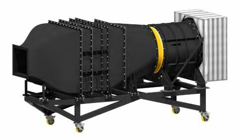
Wind tunnel configuration: Blow down Test section: Open (Jet) Engine power: 15,0 kW
