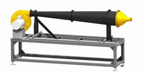
Wind tunnel configuration: Blow down Test section: Open (Jet) Engine power: 11,0 kW
