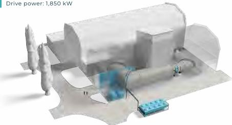
The upgrade of the entire facility required upgrades of the low-speed WT sub systems. The study also included designs of several new cooling systems proposal, an increase in power input drive, and the installation of additional equipment in the flow channel.
