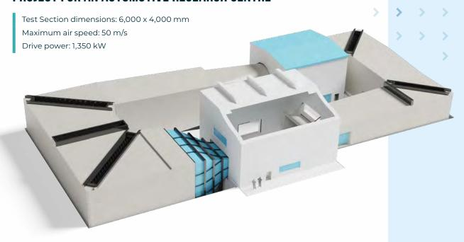
The wind tunnel project for an automotive research centre included designing the WT, implementing the design, and supervising the tunnel construction including control and measurement systems and installing the equipment.
